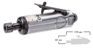
A: 6.5 м/s<sup>2</sup> Collet Size: Free Speed: 25,000 прм K: 1.1 m/s<sup>2</sup> Weight: 0.60 Kg Av Air Cons.: 4.0 CFM Noise Level: 87 DBA (98 Pwr) Output: 422 Watts
