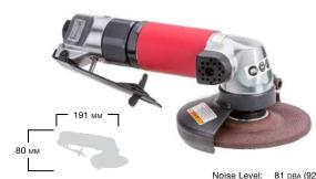
Disc Size: 100 мм Spindle Size: M10 x 1.5 Free Speed: 13,000 прм Weight: 1.04 Kg
